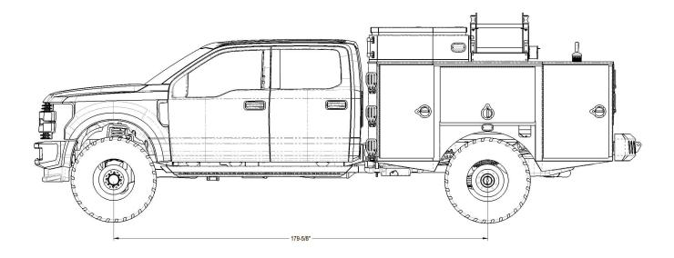
Ford® F550 , 4x4, 4 Door Chassis 6.7L 4V OHV Power Stroke V8 Turbo Diesel B20 335/80R20 Super Single Tires Darley® 1½ AGE Pump 24 HP Kubota® Hannay® Hose Reel with Electric Rewind 300 Gallon Poly Water Tank 12 Gallon Foam Cell Tomar® Emergency Light Package Smittybilt® 17.5 Winch Custom BME Console
