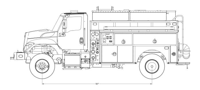
International® HV507, 2 Door, Single Axle Cummins® L9 Engine, 350 HP Allison® 3000 Transmission Darley® JMP 500, 2-Stage Pump 1500 Gallon Poly Water Tank 20 Gallon Poly Foam Tank FoamPro® 2001 Foam System
