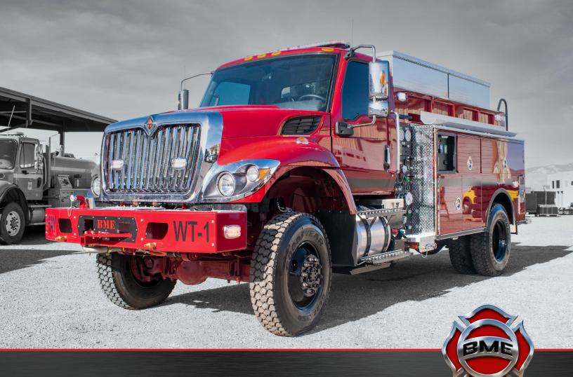
BME Fire Trucks' Tactical Tenders are designed and manufactured with the end-user in mind. With a 181-inch wheelbase and 1,500-gallon tank, this tender can maneuver through the harshest conditions while providing support on the front lines.
