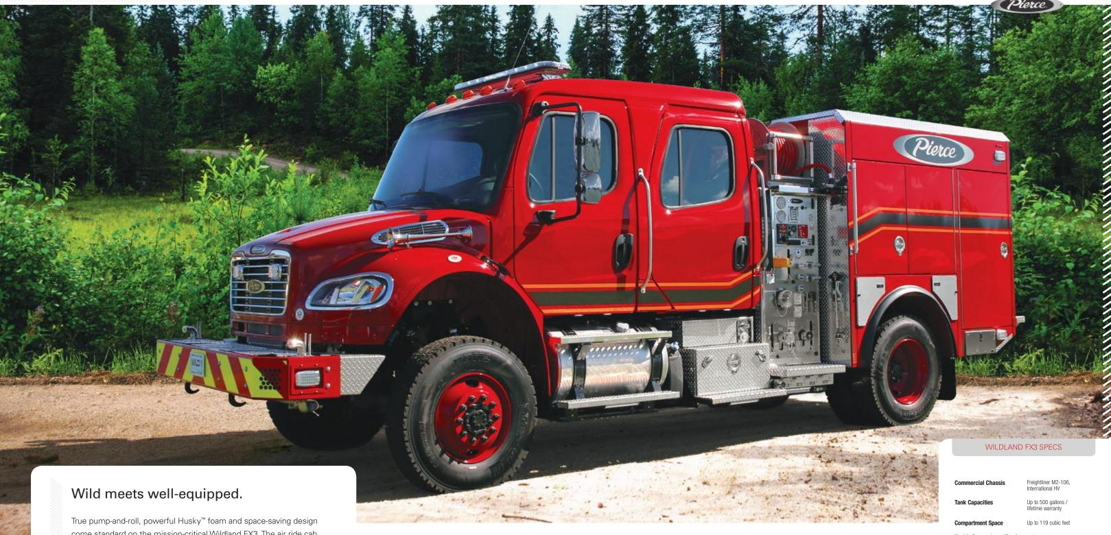
True pump-and-roll, powerful Husky™ foam and space-saving design come standard on the mission-critical Wildland FX3. The air ride cab comfortably fits 5 personnel, with a stainless steel body that integrates full-depth left side compartments, 6 standard fender compartments, lowered compartment floors, and large undercab compartments.
