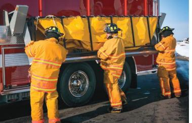
Swingdown folding tank storage. Shown on a pumper tanker.
