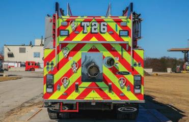
Rear dump. Shown on a pumper tanker.
