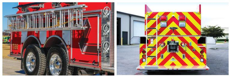
Dropdown ladder rack storage. Shown on a pumper tanker.
