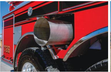
Side dump. Shown on a pumper tanker.
