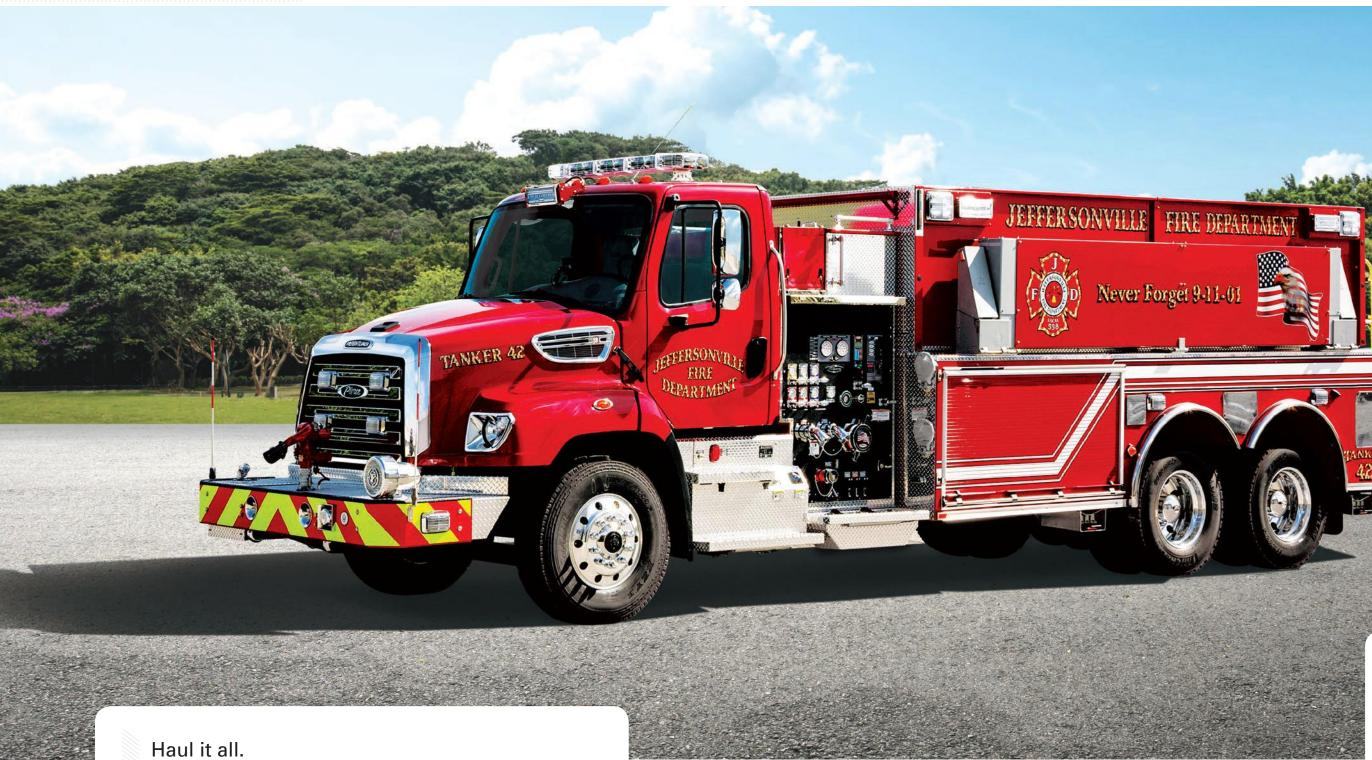
The Pierce® dry-side tanker can haul 1,800 to 4,000 gallons of water while stowing equipment on both sides and comfortably accommodating hose lines.
