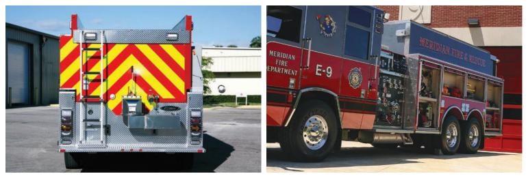
Swivel dump valve and safe access to hosebed. Shown on an FXT.
